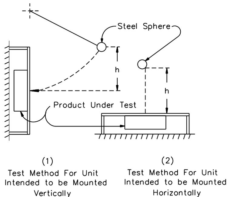
21.3 For this test, the unit is to be energized in the standby condition and connected to a rated source of supply. Following the jarring, the unit is to be tested for signaling operation.
